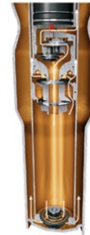
Compression in Normal mode—working piston and bypass, sporty-comfortable tuning
